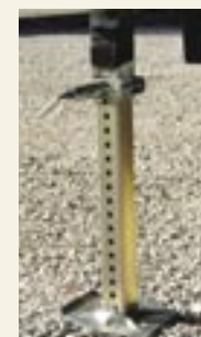
Hydraulic landing gear on Fifth Wheels (Optional) 10 times faster than conventional electric jacks. Quick release pins on Fifth Wheel feet. (Standard)
